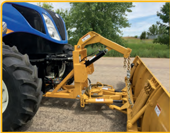
PLUG & PLAY BULKHEAD FOR QUICK DISCONNECT
